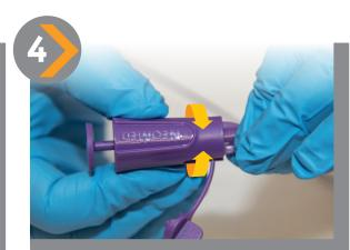
Rotate the cleaning tool to dislodge debris.
